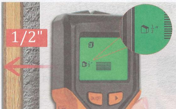
**✗** Incorrect selection of scan mode results in inaccurate detection
