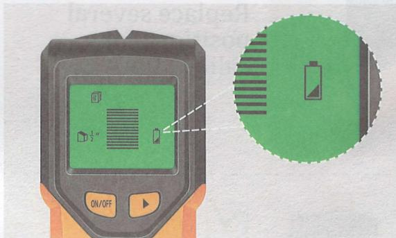
When the battery icon is displayed on the display screen, it means that the battery level is low. Detecting when the battery level is low may result in inaccurate results. Please replace the battery in a timely manner
